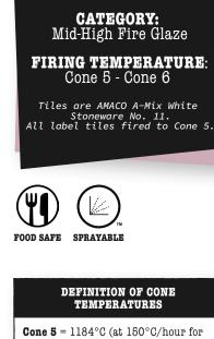
**Cone S** =  $1184^{\circ}$ C (at  $150^{\circ}$ C/nour for the final 100°C of firing) /  $2201^{\circ}$ F (at  $270^{\circ}$ F/hour in the final 200°F of firing)
